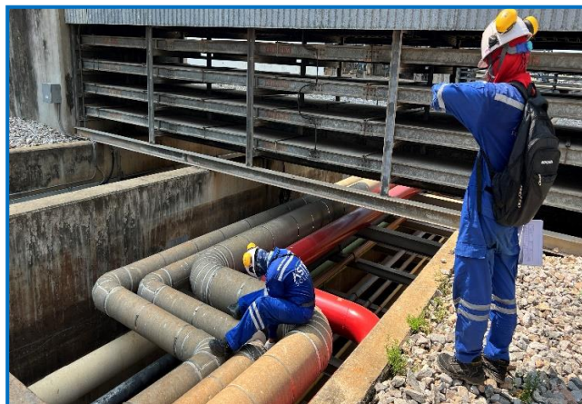
PIGTURE 1 Inspection Thickness Fuel Oil Pipe by Measurement (USTM)
